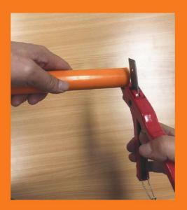
Ream the pipe by pushing the reamer into the pipe and turning. This cuts the pipe end straight while cutting chamfers on the inside and outside of the pipe end. The design of the reamer will privet shavings from falling into the pipe.
