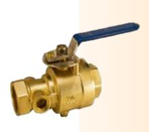
This Test & Drain Valve Used to test waterflow through sprinkler systems. When not in the closed position, the valve can be either fully open (full port),
